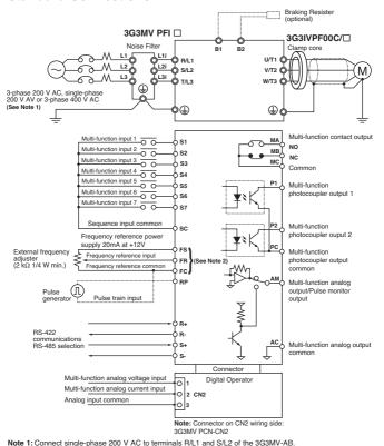
Note 2: By using pin 2 of SW2, voltage input or current input can be selected as a frequency reference input.
