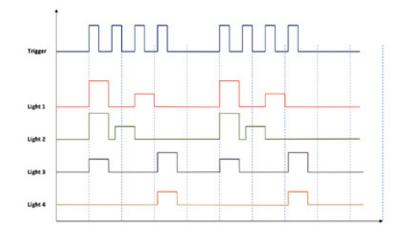
This works as in this diagram. The lighting controller is triggered once for each image to be taken. On each trigger a different combination of lights is pulsed to take four images with different lighting schemes. When the next par arrives the sequence repeats.
