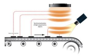
Using Pulsing, it is possible to freeze the image of moving objects. Gardasoft's controllers have fine adjustment of the pulse timing, which is often more flexible than the camera's timing. The camera can be set for a longer exposure time and the light pulsed on for a short time to freeze the motion.
