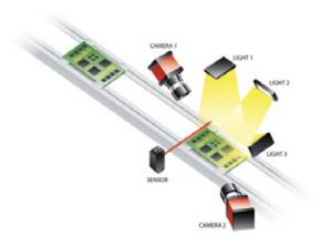
One input is used to trigger the light pulses, and another can be used to reset the sequence to ensure that the system starts in a synchronized state. An Ethernet command can also be used to reset the sequence.
